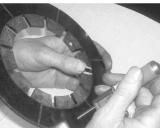
(Fig 7). **Driven Plate Measurement**
