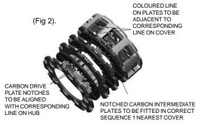
The carbon Intermediate plates are identified with notches on the outside edge (fig. 2). The plates are not all identical and must be installed in the correct sequence and
